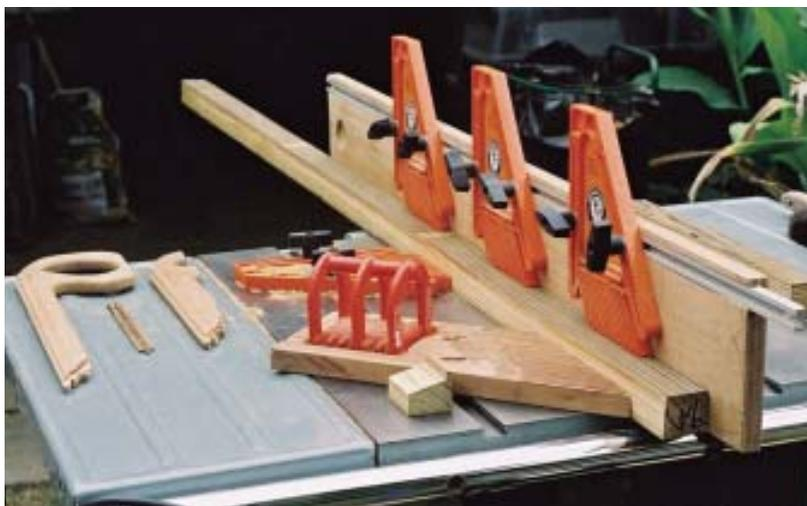
**Figure 3.** Feather boards prevent kickback and help produce better-quality saw cuts and dados. A sturdy magnet holds the shop-made wood feather board on the saw's cast-iron table. The plastic feather board mounted on the table in the miter-gauge slot and the vertical feather boards on the rip fence are made by Bench Dog Tools.
