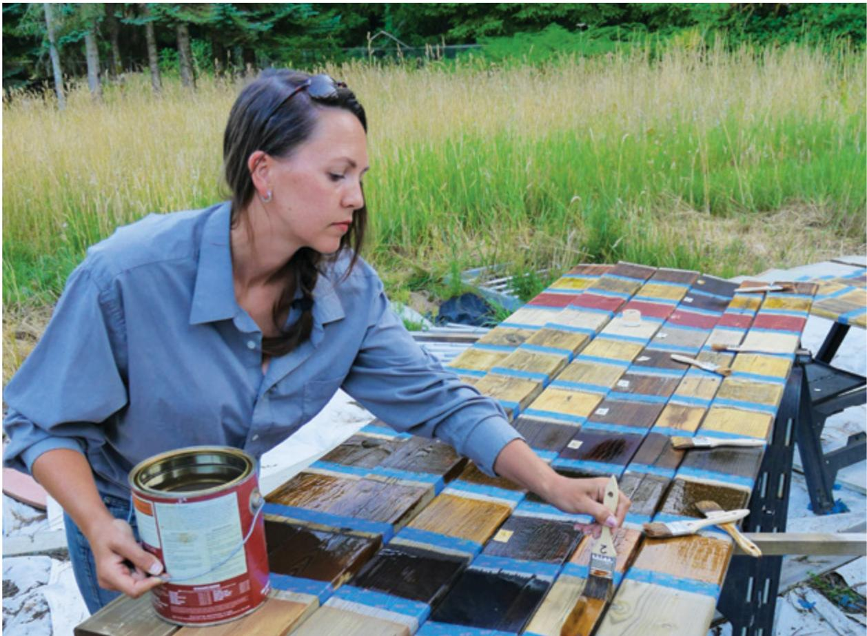
**Figure 1.** Deck boards were divided into sections with masking tape, and finish was applied to each section per manufacturer recommendations. Stains were tested on (left to right) lodgepole pine, ACQ-treated southern yellow pine, micronized CA-treated southern yellow pine, ipe, western red cedar, and ACQ-treated hem-fir decking.
