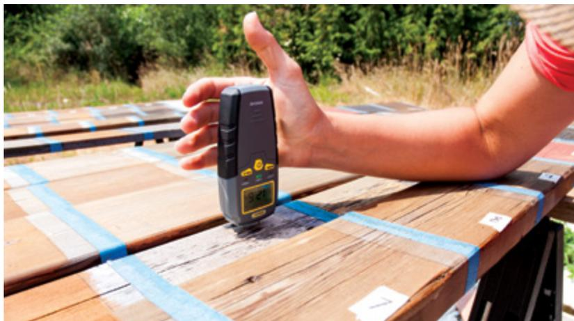
**Figure 2.** Some of the finishes did a good job of repelling moisture, even after nine months (top). Actual moisture content was tested (above) after soaking the boards for three days, then allowing them to dry for four hours. The results are noted on the chart on page 28.
