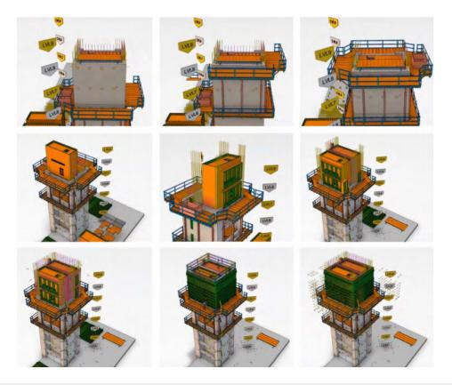
**Timber Tools** | Corrected sequence for formwork installation enabled through 3D simulation. (Photos courtesy of CadMakers)
