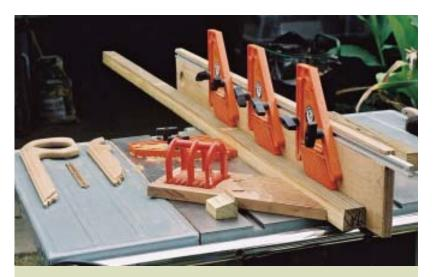
Figure 3. Feather boards prevent kickback and help produce betterquality saw cuts and dadoes. A sturdy magnet holds the shop-made wood feather board on the saw's cast-iron table. The plastic feather board mounted on the table in the miter-gauge slot and the vertical feather boards on the rip fence are made by Bench Dog Tools.
