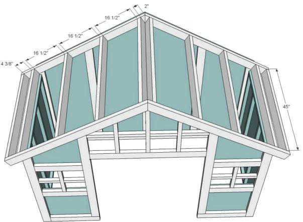
Once all the walls were built, attached the front and back walls to the side walls to create the walls of the playhouse. Then add rafters to make the roof.
