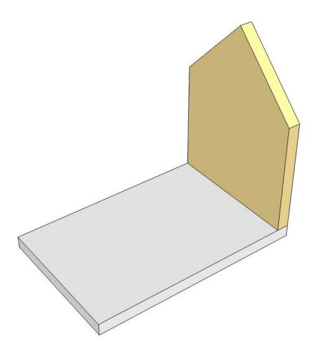
Attach the floor to the back wall, with back edges flush.
