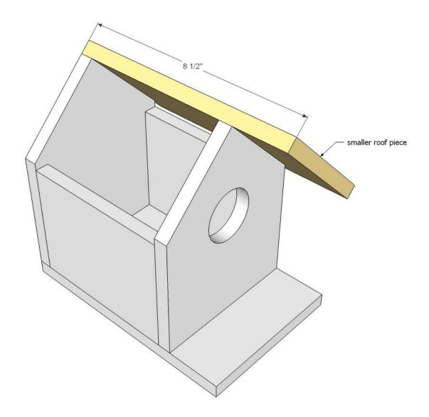
One of the roof pieces needs to be 1/2" (or thickness of the fence pickets) less in width than the other since the overlap. Rip 1/2" off one long side (cutting with the grain) on one of the roof pieces. Attach to front and back top edges.
