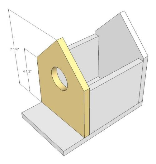
Attach front wall to sides and floor. Note that I drilled the whole afterwards with a 2" bit.
