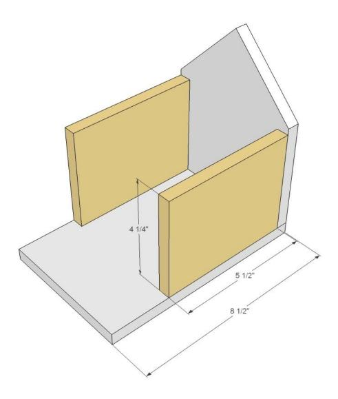
Attach side walls to back wall and floor.
