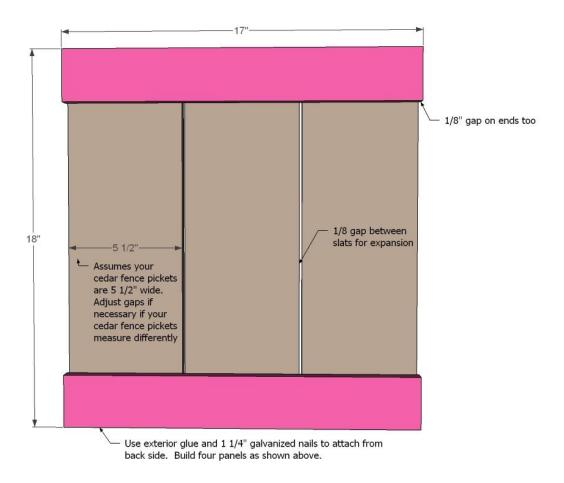
Start by building the four panels. This plan to allows for an 1/8" gap between the cedar pickets as they will shrink/ expand with moisture, and taking into account board imperfections. Use 1¼" galvanized nails and exterior glue from the insides.
