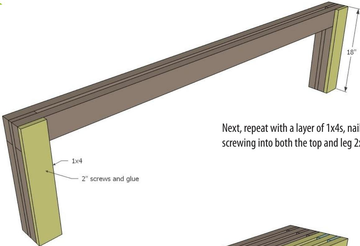
Next, repeat with a layer of 1x4s, nailing or screwing into both the top and leg 2x4s.
