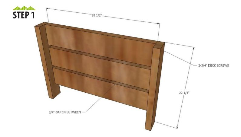
Use 2 - 2 <sup>3</sup>/<sub>4</sub>" or longer screws and exterior wood glue to attach legs to the longer 2x6 boards, with <sup>3</sup>/<sub>4</sub>" spacing in between. Recommend two screws per joint.
