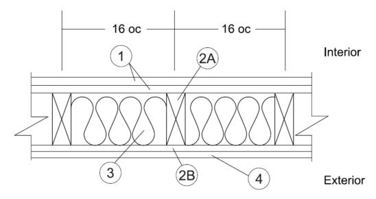
GYPSUM BOARD [Interior): Two layers Type C USG Firecode<sup>®</sup> C Core complying with ASTM C1396, min.
