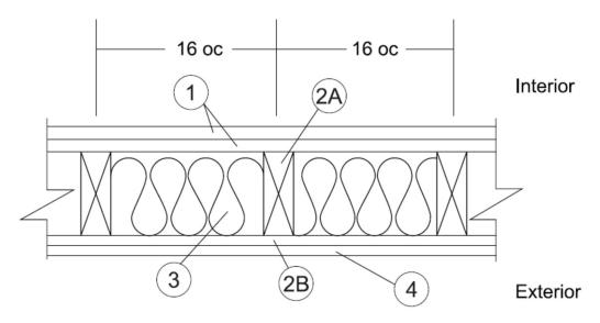
GYPSUM BOARD (Interior): Two-layers USG Firecode<sup>®</sup> C Core, complying with ASTM C1396, or equivalent, min. <sup>5</sup>/<sub>8</sub> in. thick, 4 feet wide applied vertically, fastened to framing. Face layer joints staggered with base layer and covered with paper tape and joint compound.
