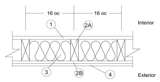
GYPSUM BOARD [Interior): One-layer Type C USG Firecode® C Core complying with ASTM C1396, minimum <sup>5</sup>/<sub>8</sub>-inch-thick (16 mm), 4 feet (1.2 m) wide applied vertically, fastened to framing. Joints covered with paper tape and joint compound.
