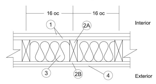
GYPSUM BOARD [Interior): Two layers Type C USG Firecode® C Core complying with ASTM C1396, minimum <sup>5</sup>/<sub>8</sub>- inch-thick (16 mm), 4 feet (1.2 mm) wide applied vertically, fastened to framing. Face layer joints staggered with base layer and covered with paper tape and joint compound.
