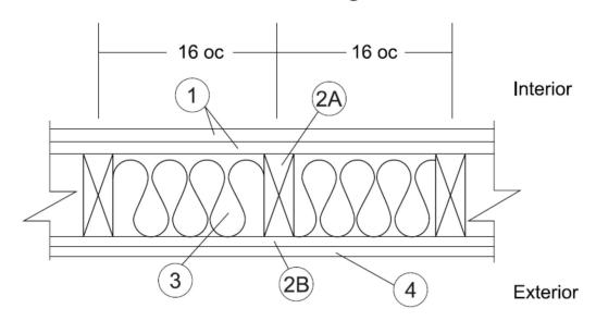
1. GYPSUM BOARD (Interior): Two-layers USG Firecode<sup>®</sup> C Core, complying with ASTM C1396, or equivalent, minimum <sup>5</sup>/<sub>8</sub>-inch-thick (15.69 mm), 4 feet (1.2 mm) wide applied vertically, fastened to framing. Face layer joints staggered with base layer and covered with paper tape and joint compound.
