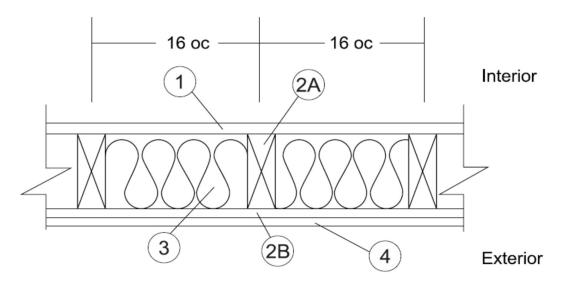
GYPSUM BOARD [Interior): One-layer Type C USG Firecode® C Core complying with ASTM C1396, minimum <sup>5</sup>/<sub>8</sub>-inch-thick (16 mm), 4 feet (1.2 m) wide applied vertically, fastened to framing. Joints covered with paper tape and joint compound.
